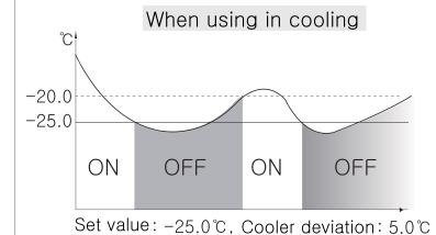
Current value > Setting value + Cooling deviation Output ON
