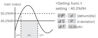
ex) Humidifier → turn off at 50%RH,turn on at 40%RH How to operate(setting for the humidity & programs)?
